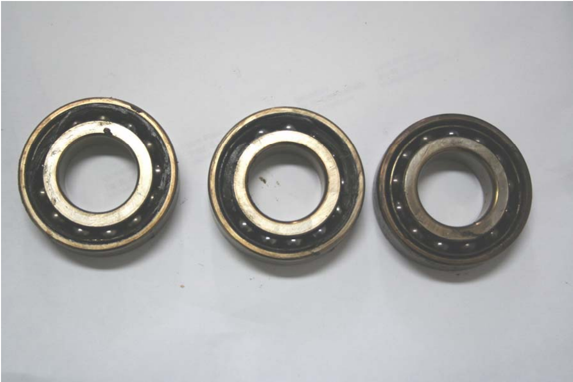
Figure 12: Test Bearings after test showing caky black grease
