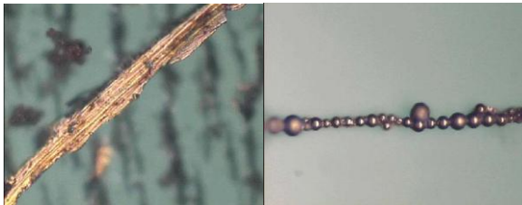
Flat elongated platelets (Excessive load/speed on sliding surface) Small sphere (Rolling contact failure)
