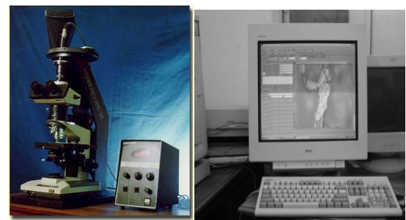
Importing image captured in the Ferroscope to computer for comparison
