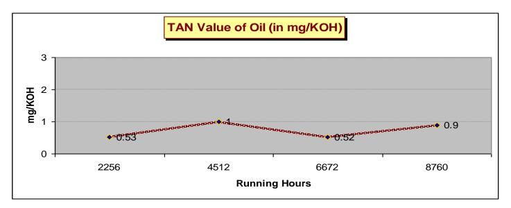
The TAN value of the oil was also monitored on a quarterly basis. As can be seen from the test data, the there has been almost no rise in the TAN value even after 6672 hrs of operation. The change in TAN value if only 0.45 after 1 year (8760 hrs).
