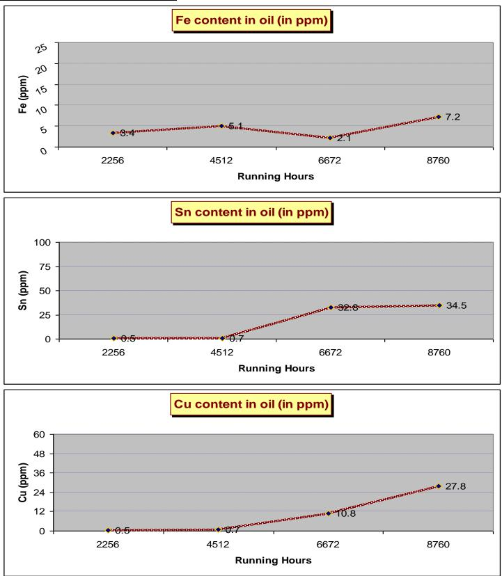
The wear debris analysis shows that there has been very minimal wear and tear during the first one year of operation, i.e 8760 hrs. There has been an increase in the value of wear metals in the sample after running for more than 6672 hrs. This is normal for oil which has been in operation for prolonged continuous use for such a long time.
