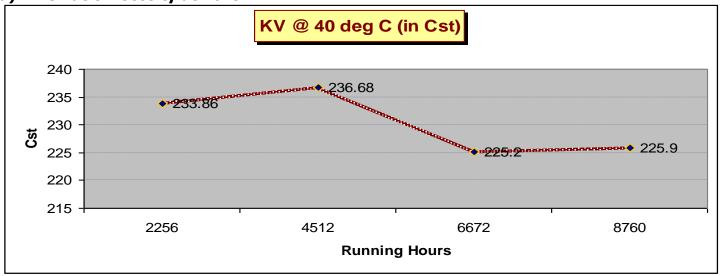
The oil was first tested after 2256 hrs into operation. The Kinematic Viscosity at  $40^{\circ}$ C was found to be well within the limits. The oil samples were subsequently tested at various running hours as shown above. The test data
